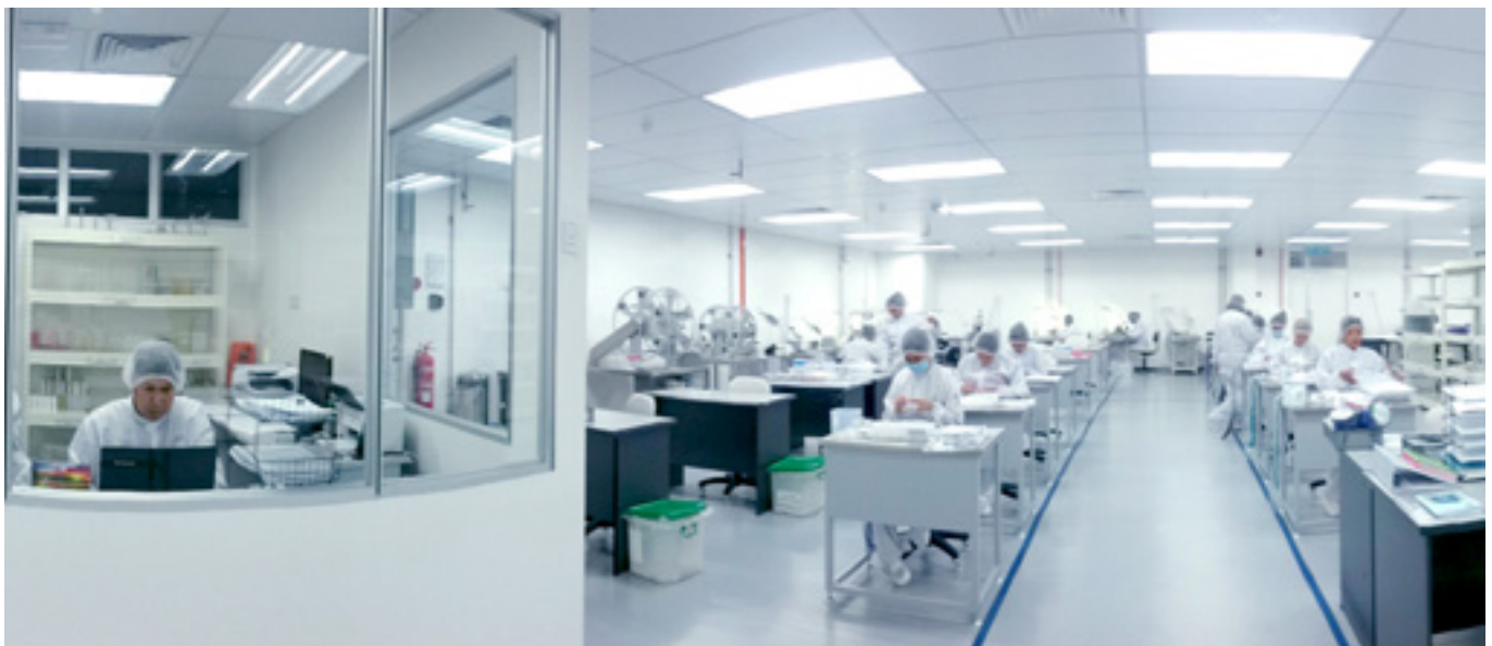
Vigilenz's ISO Class cleanroom manufacturing area compliant to ISO 13485:2016, equipped with in-house microbiology laboratory.
